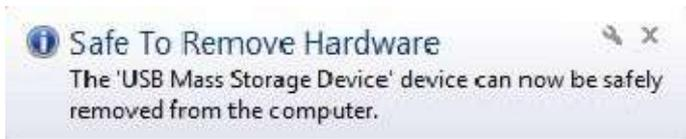
, indicates the U disk pull out from computer successfully. Now user can insert the U disk to the controller to start the file operation.
